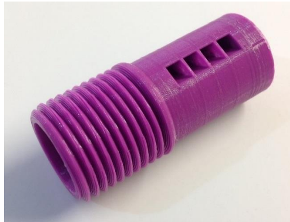
Figure 5. Variant of the mesh nozzle diaphragm. Source: authors' development.
