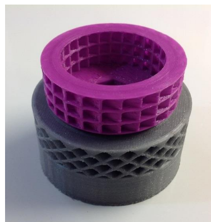
Figure 13. Micromodel of the mesh turbine rotor according to RF patent No. 203,833 (variant). Source: authors' development.
