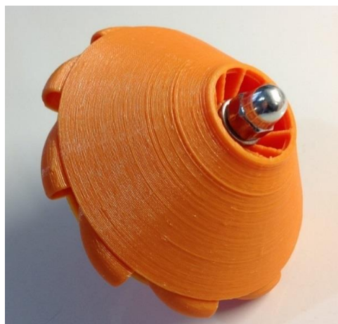
Figure 3. Micromodel of Euler turbine (rotor version). Source: authors' development.
