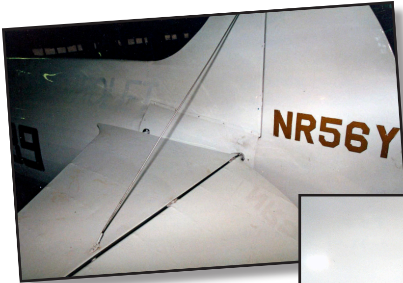
Bottom elevator guy wires are also simply bolted and tightened with threaded ends.
