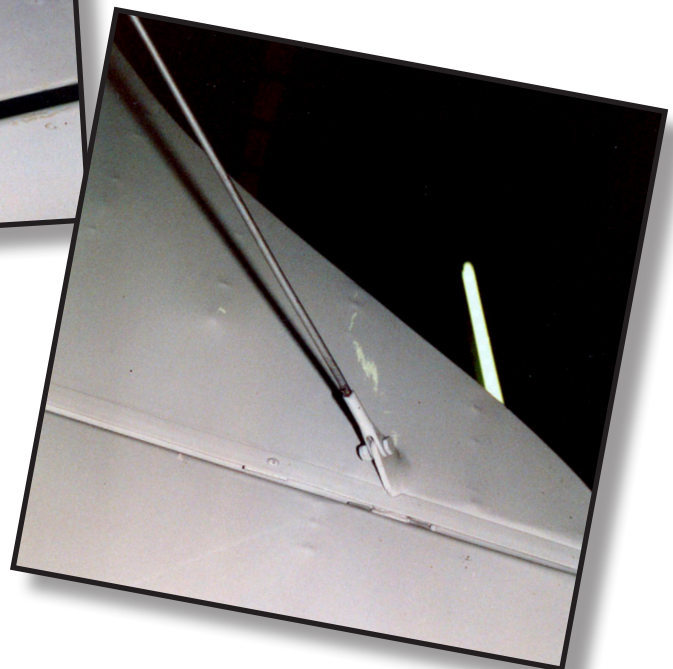
Bottom elevator guy wires are also simply bolted and tightened with threaded ends.
