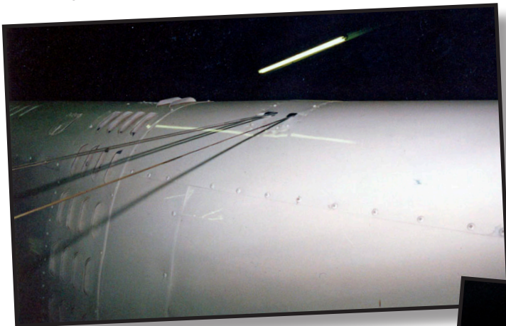
Wing guy wires terminate inside the top of the nose cowling.
