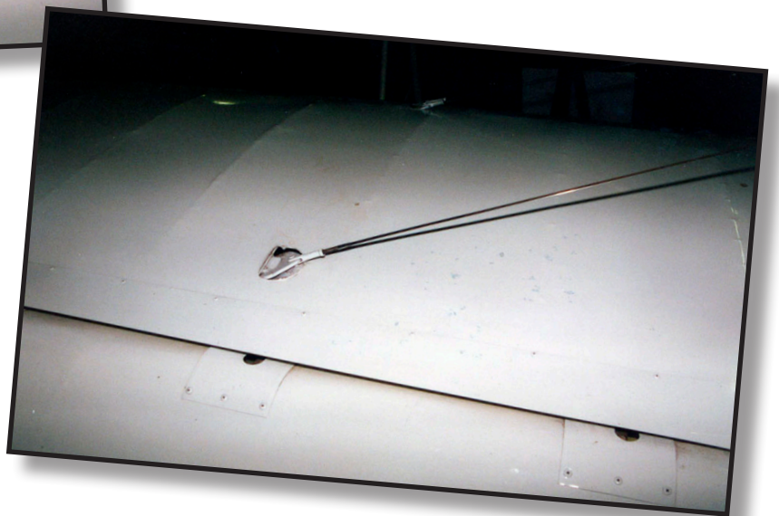
Aft left wing guy wires also terminate inside the wing.
