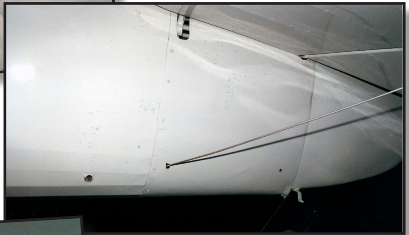
Bottom elevator guy wires are also simply bolted and tightened with threaded ends.
