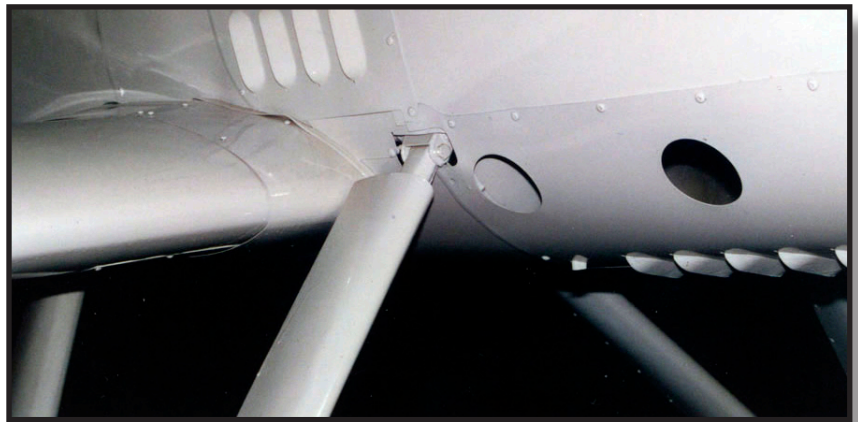
Right front wing root with details around the landing gear.
