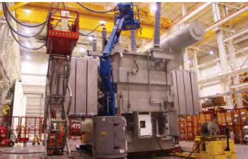
420 MVA top-rated, 345 kV autotransformer is ready for test in Waukesha's manufacturing facility
