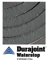
Durajoint EXPAND-Tite is a flexible concrete construction joint waterstop that is easy to install in non-moving joints. It is composed of bentonite clay and butyl rubber to withhold its physical integrity after expanding.
