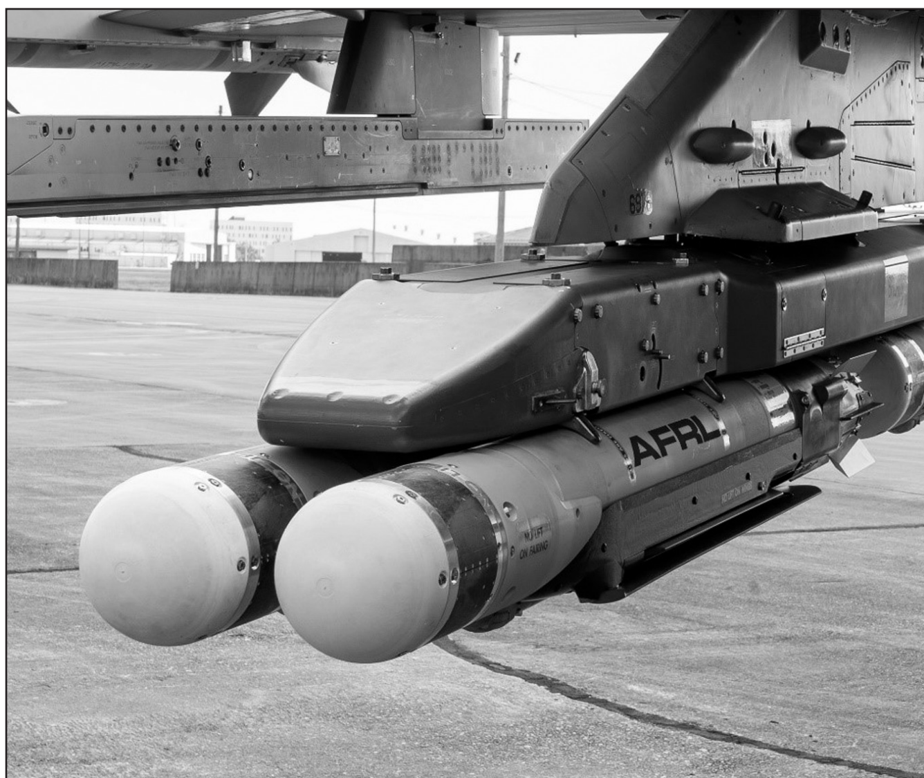
Four Collaborative Small Diameter Bombs hang from the wing of a 96th Test Wing F-16 fighter. Two of the bombs were dropped during the first flight demonstration of the Air Force Golden Horde Vanguard. (Courtesy photo)
