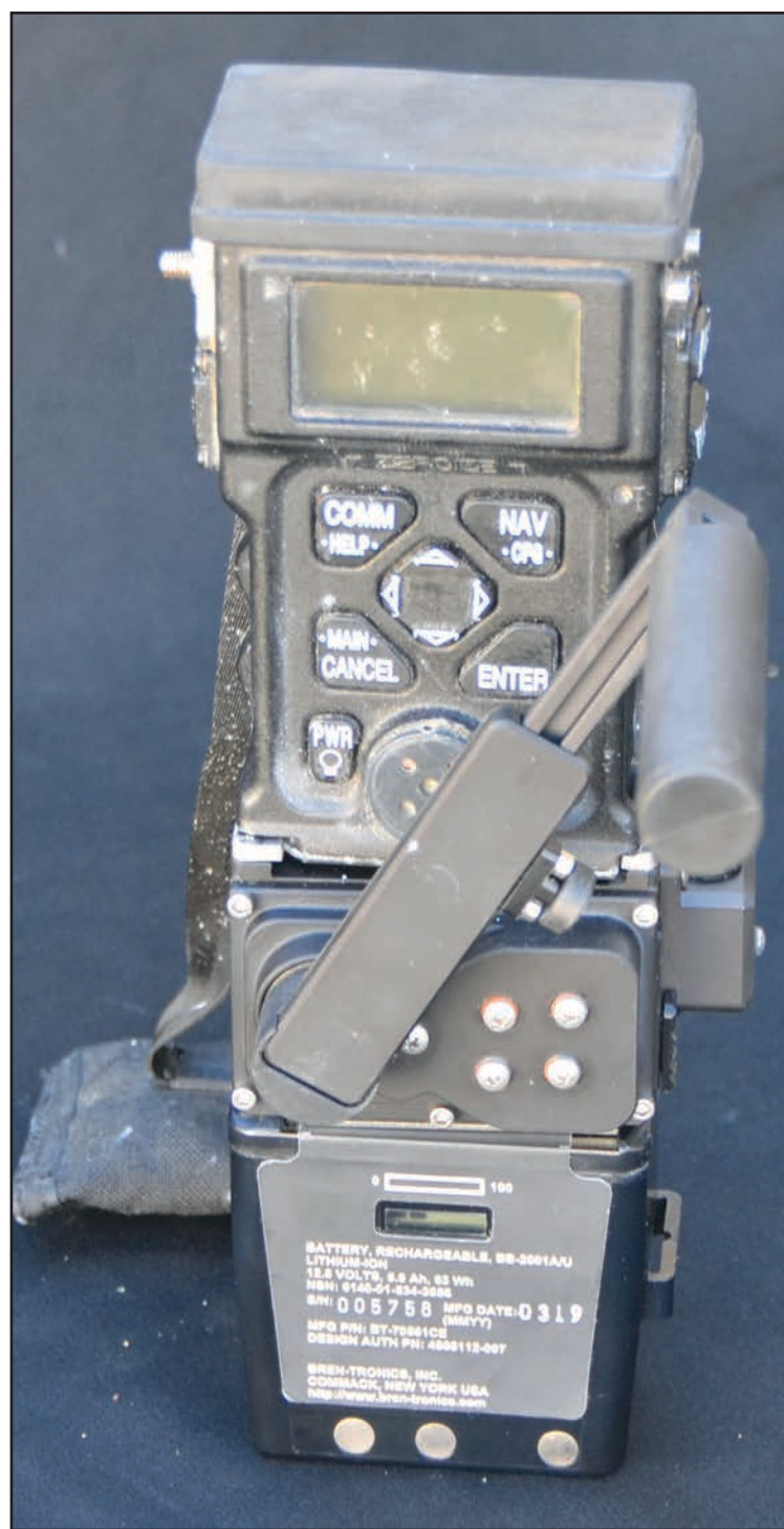
A removable hand-crank provides on-the-go power to the Surge charging device, shown here with the Combat Survivor Evader Locator radio, top, and battery, bottom, all connected. (Photo courtesy of Combat Power Solutions, LLC)
