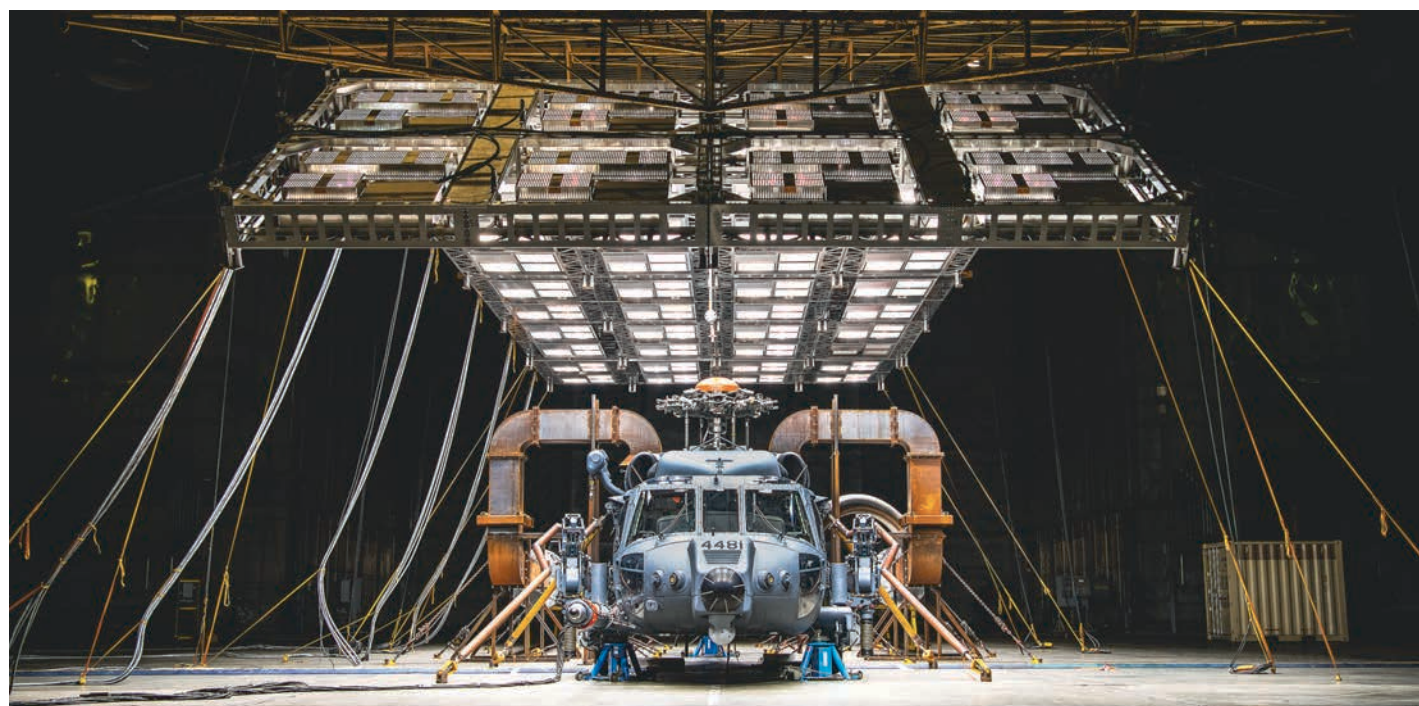
An HH-60W Jolly Green II sits under bright lights used to create heat in the Arnold Engineering Development Complex McKinley Climatic Lab March 19 at Eglin Air Force Base, Fla. The Air Force’s new combat search and rescue helicopter and crews experienced temperature extremes from 120 to minus 60 degrees Fahrenheit as well as torrential rain during the month of testing. The tests evaluate how the aircraft and its instrumentation, electronics and crew fare under the extreme conditions it will face in the operational Air Force. (U.S. Air Force photo by Samuel King Jr.)
