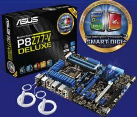
LGA1155 socket for Intel® 3rd/2nd Generation Intel® Core™ processor family / Intel® Z77 Chipset
