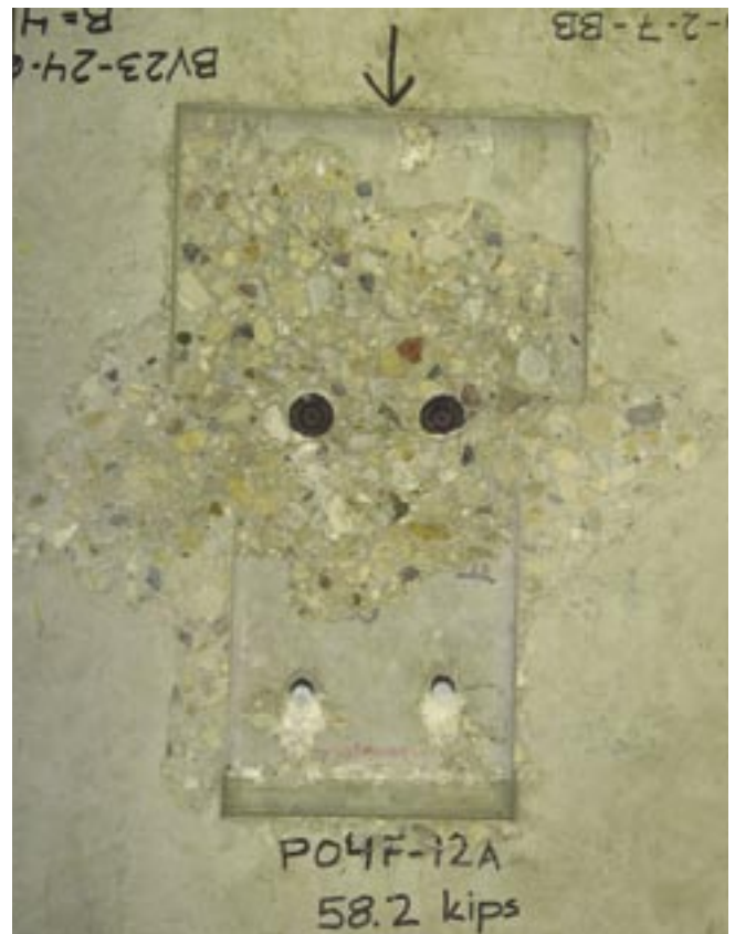
Fig. 12. Mixed mode failure of Test PO4F-12A with y = 6 in. (152 mm) showing steel failure of front studs and concrete breakout at the rear studs.
