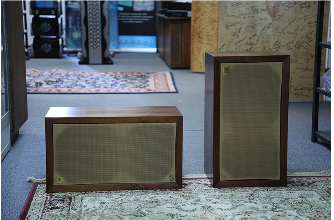
Spotted at Audio Classics: Acoustic Research AR-3 loudspeakers. The AR-3 premiered in 1958 and features the first production dome tweeter and midrange driver, plus a 12-inch cone woofer.
