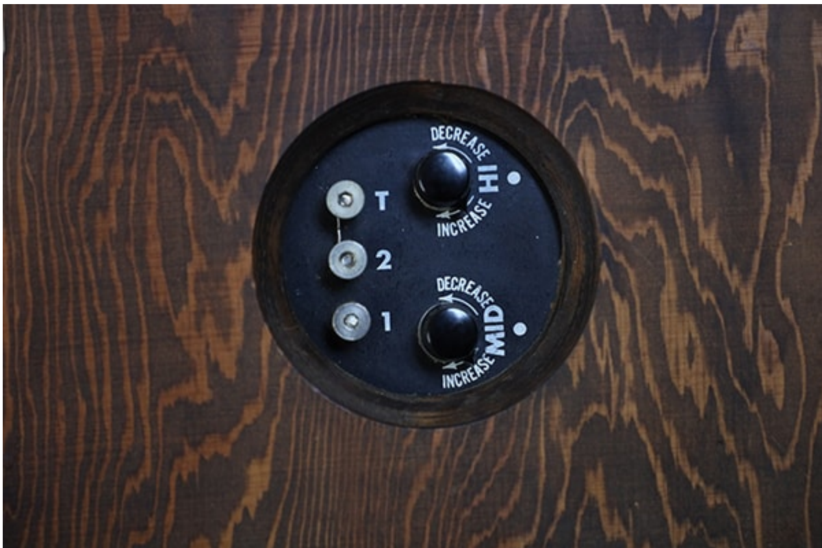
One of the coolest-looking sets of speaker-level controls ever. AR-3, rear panel.
