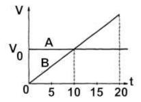
At time t = 0, car A traveling with speed  $v_0$  passes car B, which is just starting to move. Both cars then travel on two parallel lanes of the same straight road. The graphs of speed v versus time t for both cars are shown above.
