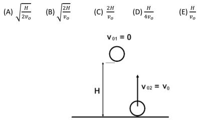
38. A ball is dropped from a height H a second ball is thrown from the ground with an initial velocity v<sub>o</sub>. How fast does the first ball move when they pass each other?
