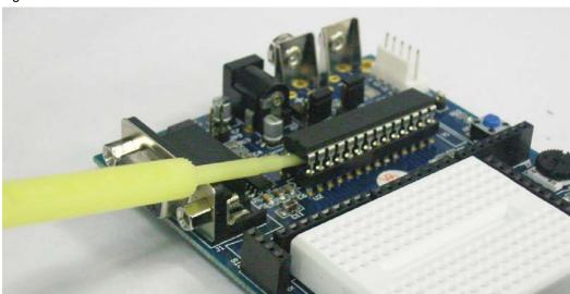
Place the CY8C27443-24PXI silicon on the IC socket. Ensure that the silicon notch is aligned with the notch on the IC socket; see Figure A-6. Press down gently to finish the replacement.
