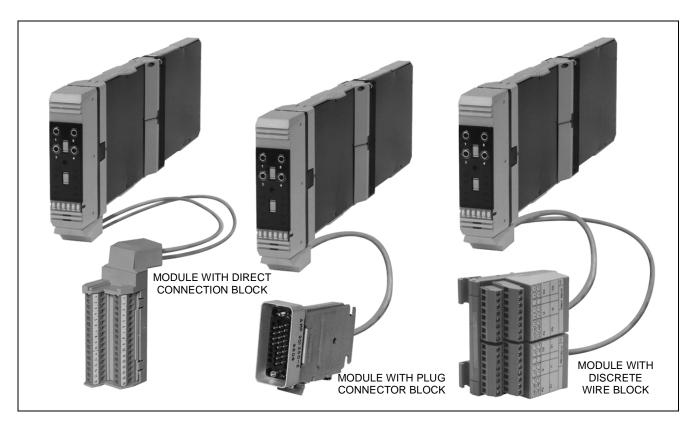
The Intelligent Transmitter/0 to 20 mA Output Interface Module contains four Intelligent Transmitter interface channels and four 20 mA dc analog output channels. The module is a main type and independently connects to the redundant Fieldbus.
