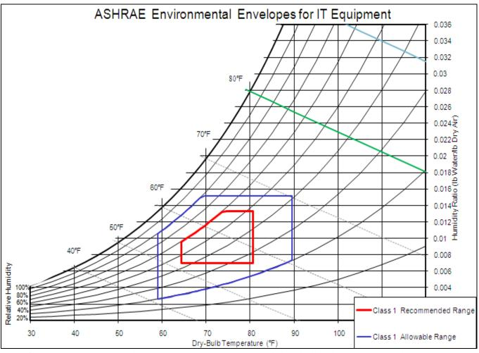
*Figure 1 Psychrometric chart showing ASHRAE recommended and allowable environmental envelopes for IT equipment.*<sup>2</sup>(Source: Ian Metzger, NREL)
