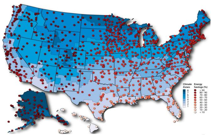
*Figure 4* Energy savings potential for recommended envelope, Stage 2: Economizer + Direct Evap. Cooling.<sup>15</sup> (Source: Billy Roberts, NREL)
