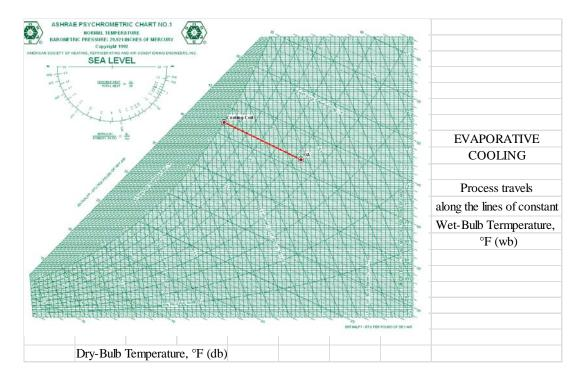
The next thing to address is when you do not want to add moisture. Then you would only want to do Sensible Cooling, which involves dropping the temperature but neither raising nor lowering the moisture content of the air. If you do not take out or add any moisture and you drop the temperature, the relative humidity will increase. Relative Humidity is the ability of the air to hold moisture in relation to the temperature of the air.
