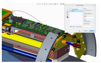
Determine the connections either manually or from logical information. PTC Creo PCX automatically generates a simple path which then enables the user to find the optimum path faster.
