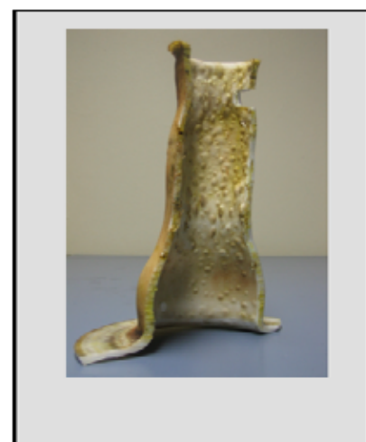
Typical permeation failure of isostatically formed liner
