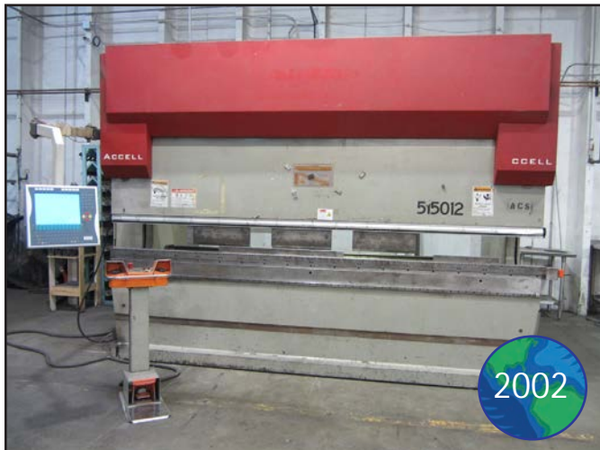
ACCURPRESS ACCELL 150 TON X 12' 6-AXIS APPROX. CNC HYDRAULIC PRESS BRAKE WITH WILA
