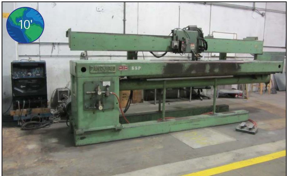
PANDJIRIS 120E9-36 10' HORIZONTAL SEAM WELDER
