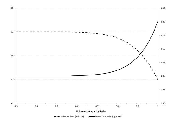
Figure 9: Relationship between volume-to-capacity ratio and travel speeds for simulation model
