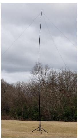
In this deployment the top two sections of the mast had been removed and the resulting top of the mast is at 34 feet. The inverted V antenna was anchored so that the wire pulled the mast in one direction. A guy rope was then attached to counter this pull, resulting in a reasonably stable installation. The mast sits on an MFJ tripod. A role-up J-pole antenna made of 450-ohm open line, with RG-8X coax can be attached at the 25-foot level of this mast for VHF/UHF operations.
