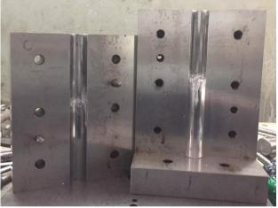
Fig2.Compaction of powder and green compact
