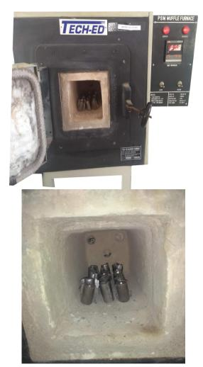
Fig3. Muffle furnace and Sintering of specimens
