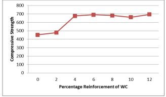
Fig5. Compressive Strength v/s Percentage Reinforcement WC
