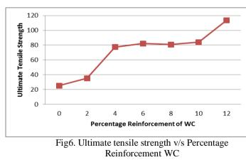
Tensile test results indicated a significant increase in Ultimate Tensile strength of 77% in MMCs when compared with base alloy.
