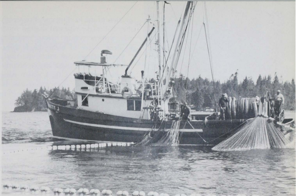
Figure 8.—Drumming continues at high speed after the table has been turned because it is not necessary to walk rings aft. Ring bridles and web moving across the narrow space between fairlead and stripper tend to inhibit fish from taking the potential escape route under the vessel.
