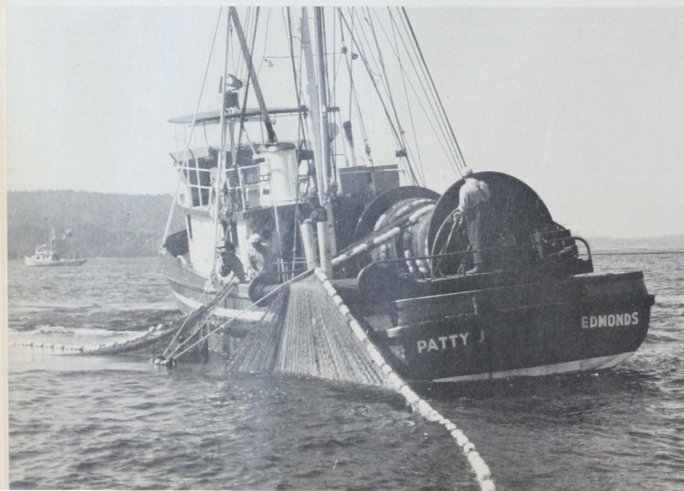
Figure 3.—The Patty J. is equipped with a hydraulically-driven pivoting drum and table to follow the changing angle to the net during retrieval and to reduce the opening between net ends.
