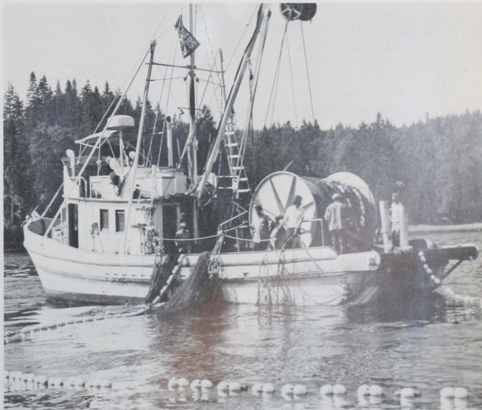
Figure 5.—After pursing is complete, rings are threaded onto a stripping device, then lifted high enough to bring the web clear of the water. Note one fisherman, holding the net out of the water, walks the rings aft to the fixed drum.
