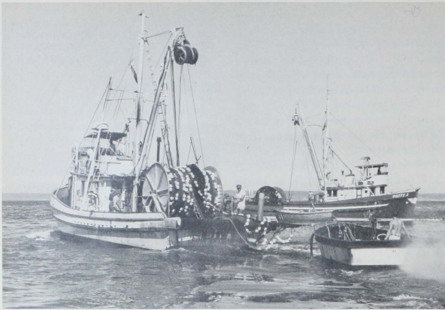
Figure 2.—The Finn has a fixed-net reel attached to the main deck whereas the reel of the Patty J. has been recessed into the deck; the latter also has a pivoting feature. Note that both vessels carry power blocks used earlier in the season when fishing Alaskan waters.
