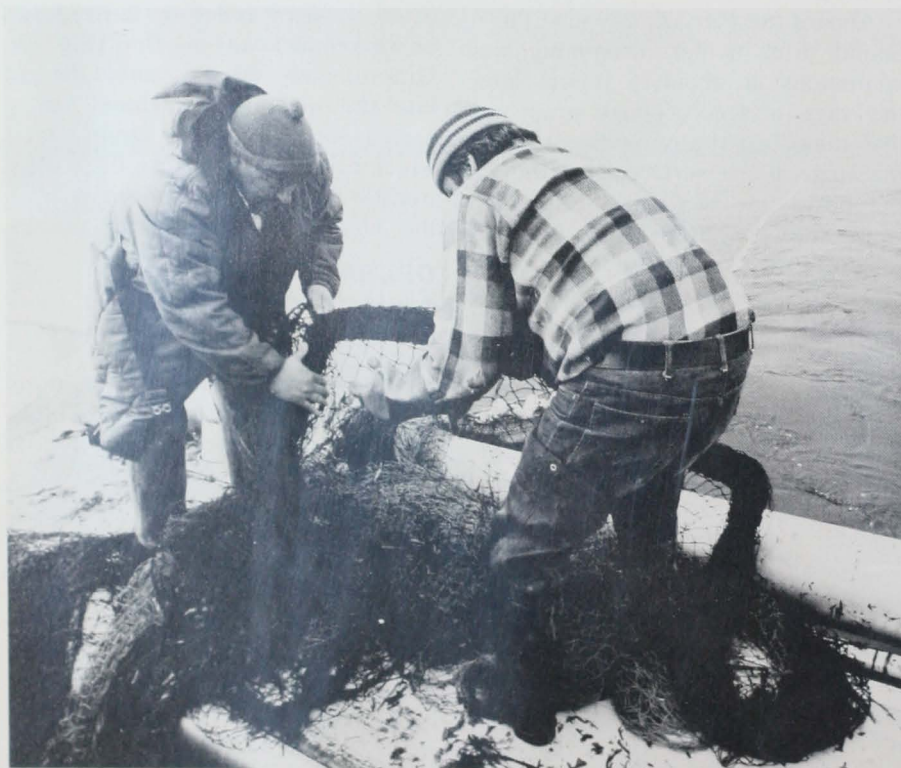
Figure 10.—Fishermen aboard the drum seiner Patty J. work in the confined space between the drum well and stern to clear a web rollup.
