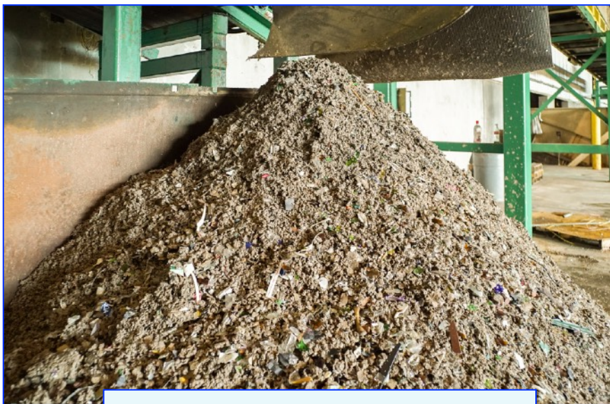
Raw Organic Fraction from the PulpStar's integral Trommel Screen
