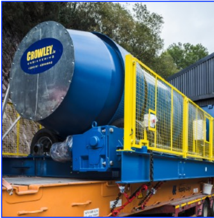
PulpStar 5 on flatpack ready for shipping. Capacity 5 tonnes per hour MSW
