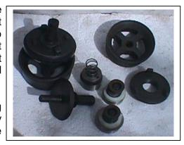
The lower valve stem with flat end facilitates holding in the vice for insert replacement without damaging the guide area. The face as well as diameter of the valve body is threaded. Both threads on valve body are coated with anti-seize compound to prevent corrosion. This facilitates replacement of insert.
