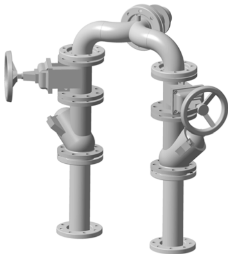
Fig. 6 DC, pipe system with direct, common outlet
