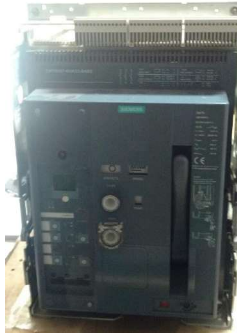
Air Circuit Breaker 3WT
