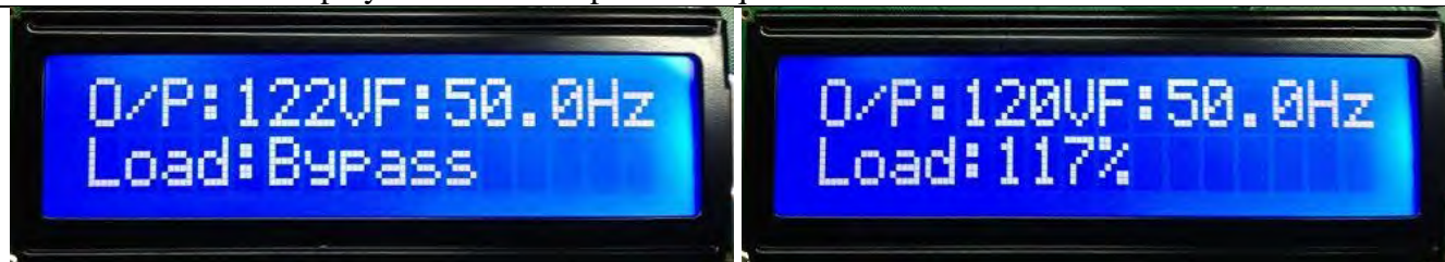
Output Voltage/Frequency and Output Current( in percentage) in Inverter mode
