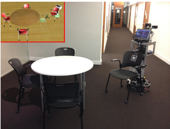
Fig. 10 A snapshot from one of the real world tests, where the task of the robot is to arrange the chairs around the round table. Visualization of the setup in simulation is provided on the top left corner of the image.
