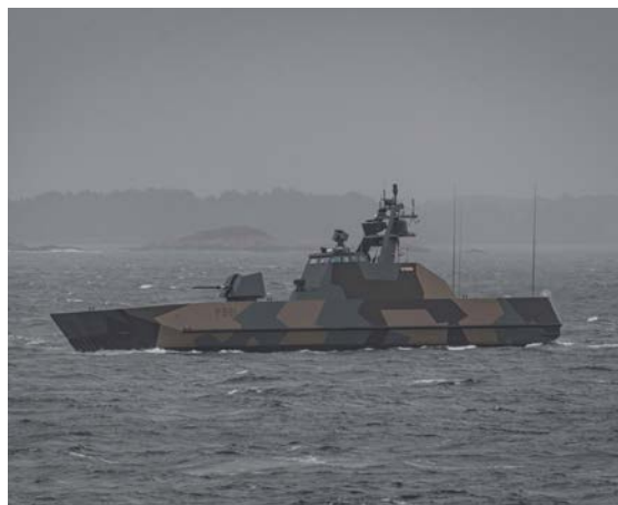
The Royal Norwegian Navy Corvette HNoMS Storm took part in the NATO exercise. This Skjold-class Corvette is a large, superfast, stealth missile corvette which specializes in littoral warfare. Capable of 60 knots, it is one of the fastest warships in the world.
