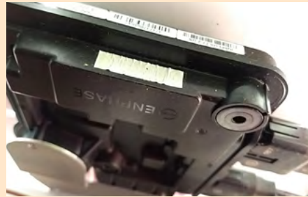
Figure 55. AC modules and micro inverters are small inverters installed integral to or adjacent to individual PV modules.
