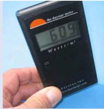
Figure 102. Handheld solar meters use a small PV cell to measure solar irradiance.
