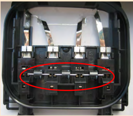
Figure 51. Bypass diodes are often located in module junction boxes.
