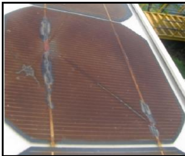
Figure 28: Corrosion marks on Bush bars and interconnects (Source: (Rajiv Dubey, 2014))
