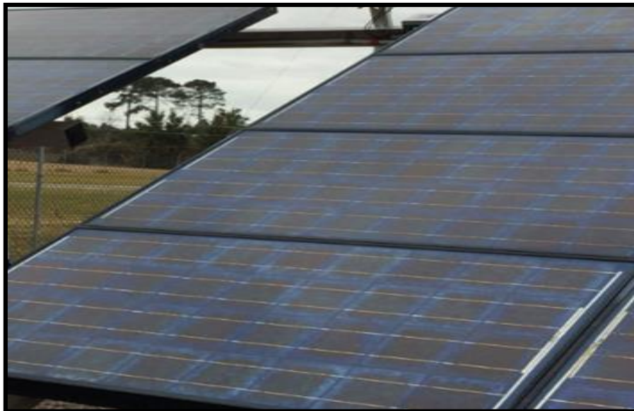
Figure 29: Discoloration shown in the solar cell of the PV module. (Source: Photo taken at Murdoch University, Perth on October 2014)
