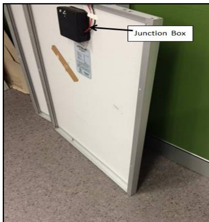
Figure 13: Junction Box in PV module (Photo taken at Renewable Lab, Murdoch University, November, 2014)
