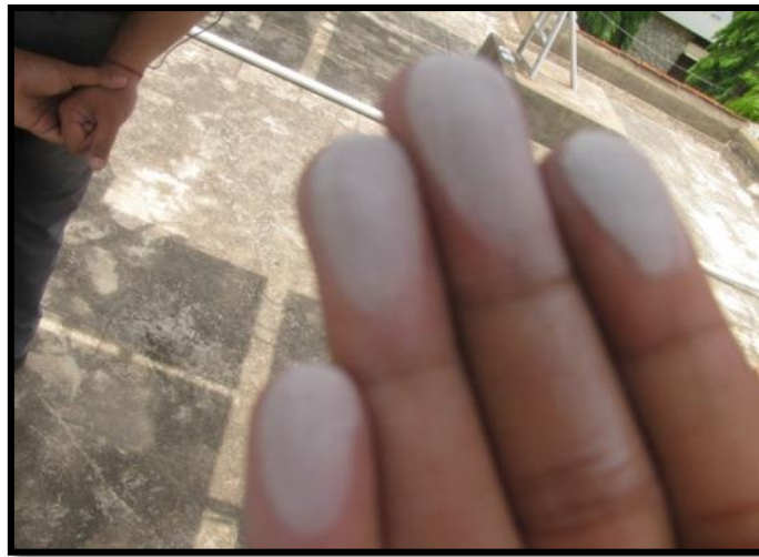
Figure 34: Chalking of the Back sheet of PV module (Source: (Rajiv Dubey, 2014))
