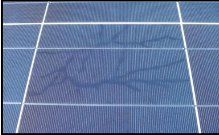
Figure 41: Snail Trails on PV module (Source: (Vashishtha, 2014))
