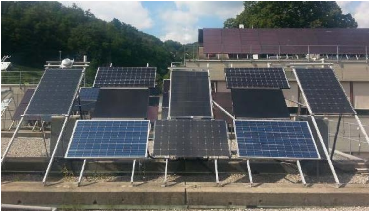
Figure 43: Test stand with different technologies, including bifacial modules at top left and top right
