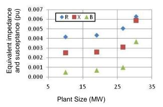
Figure 3 – Sample equivalent collector system data (R, X, B) in per unit on 100 MVA, 34.5kV base, as a function of plant size
