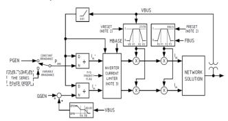
Figure 8 – Proposed model structure for distributionconnected PV
