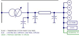
Figure 7 – Composite Load Model with PV Component
