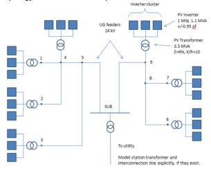
Figure 2 – Sample PV system topology
