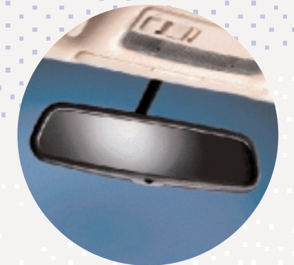
The automatic dimming interior rear-view mirror darkens if a following car's lights are too high.
