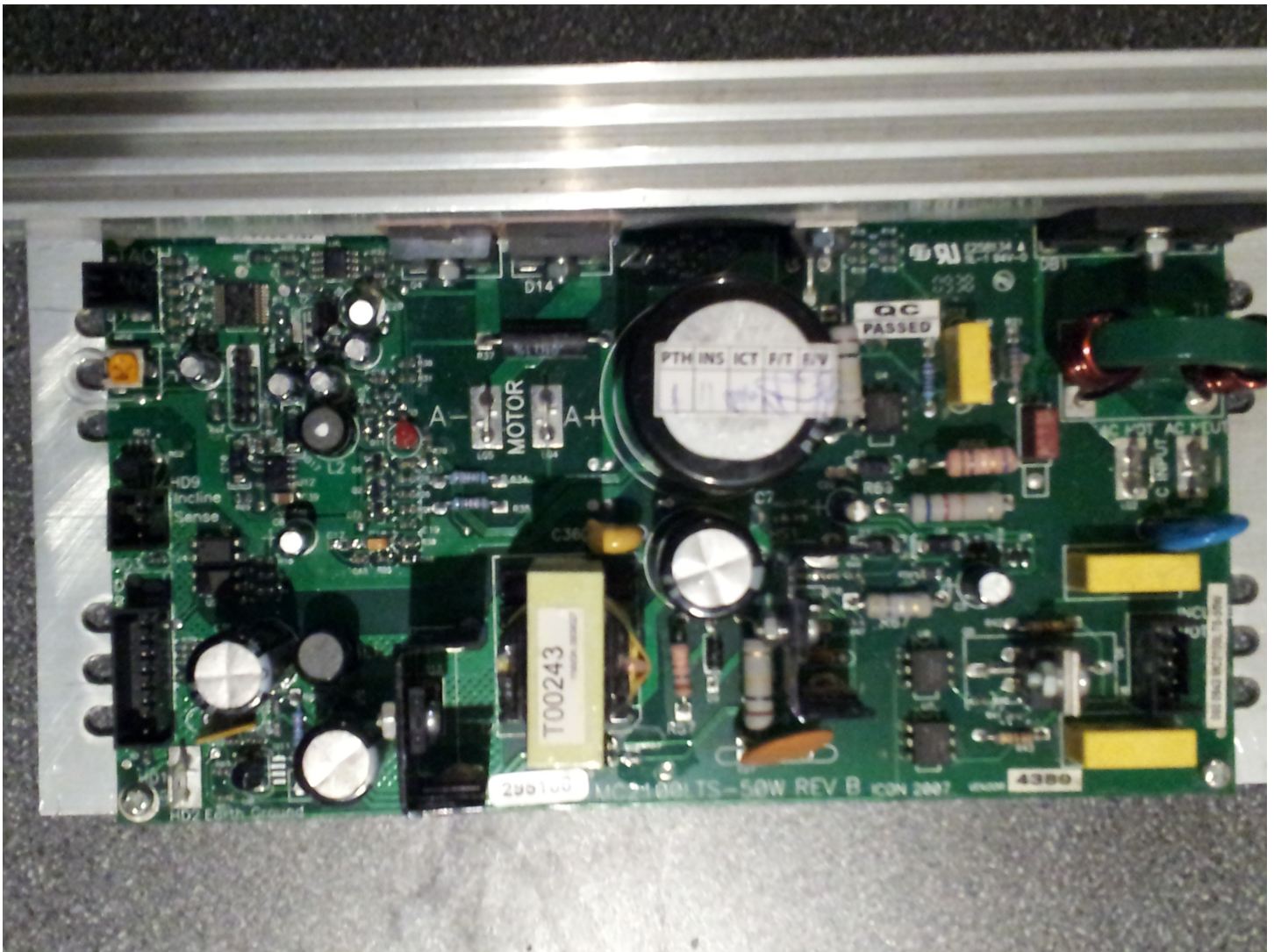
Figure 1 : MC-2100 Motor Controller Board
