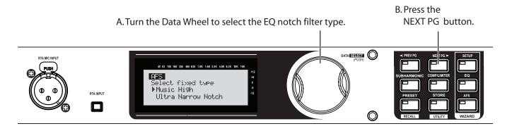
**30.** With the channel faders down, set the mixer's master level to zero (0). With the microphones you'll be using during the performance in place and connected, turn up microphone channel levels until feedback begins. The AFS will start to populate the Advanced Feedback Suppression fixed filters.
