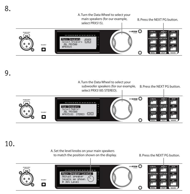
(Note that you also have the option to turn the Data Wheel to adjust the level shown on the display to match a preferred setting on your speakers.)
