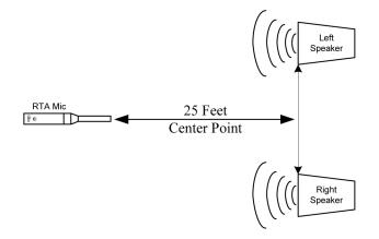
17. Turn the Data Wheel until pink noise is playing through your speakers at performance level (the same volume you intend to use during your performance). The words "SET TO PERFORMANCE LEVEL" will appear in the display when you have passed the minimum threshold. Set level higher as needed.
