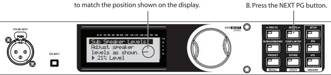
(Note that you also have the option to turn the Data Wheel to adjust the level shown on the display to match a preferred setting on your speakers.)
