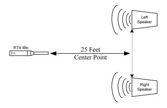
**15.** Turn the Data Wheel until pink noise is playing through your speakers at performance level (the same volume you intend to use during your performance). The words "SET TO PERFORMANCE LEVEL" will appear in the display when you have passed the minimum threshold. Set level higher as needed.
