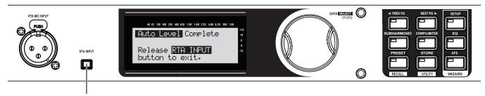
Press the RTA INPUT button to release.
