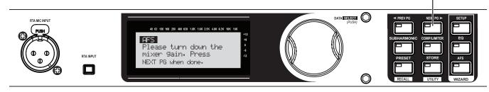
26. Turn the Data Wheel to choose the number of fixed filters to use with Advanced Feedback Suppression. These filters, once populated or FIXED, will stay at the set frequency and level. LIVE "L" filters will change as needed during a performance.
