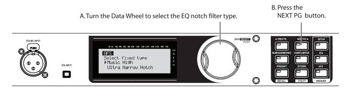
28. With the channel faders down, set the mixer's master level to zero (0 dB). With the microphones you'll be using during the performance in place and connected, turn up microphone channel levels until feedback begins. The AFS will start to populate the Advanced Feedback Suppression fixed filters.
