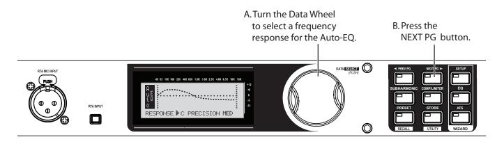
21. Turn the Data Wheel until pink noise is playing through your speakers at performance level. The words "SET TO PERFORMANCE LEVEL" will appear in the Display when you have passed the minimum threshold. Set level higher as needed. Press the <Next pg> button to continue.
