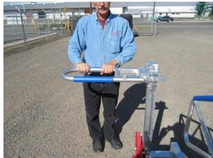
3. Once movement is complete, reengage braking mechanism by releasing the handle and allowing it to rise to the vertical position.
