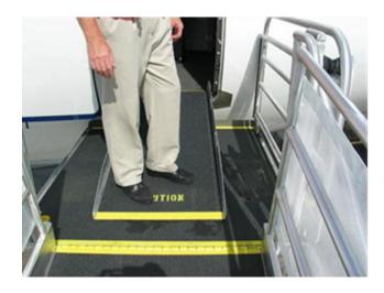
Example of deployed transition plate
