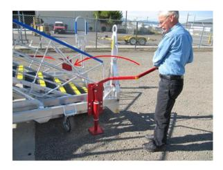
5. The stabilizer will unlock and lower the rear swivel wheel to the ground.
