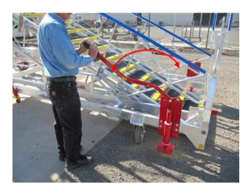
2. The stabilizer will lift the rear swivel wheel off the ground and lock into place once it has been fully engaged.
