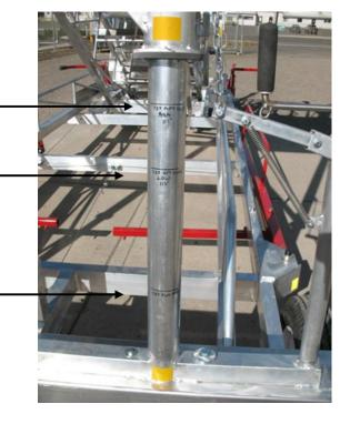
4. The Adjustment Handle has a built in limiting device to prevent the stairs from being raised too far. When the handle comes in contact with the rising bar, it has reached max height, as shown below
