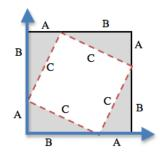
By moving the gray triangles, it is possible to create two rectangles that fit inside the original square. While the space taken up by the triangles has shifted, it hasn't gotten any bigger or smaller. Likewise, the white space has been broken into two smaller squares, but in total it remains the same size. By using the side-lengths A and B, one can calculate the area of the two squares.
