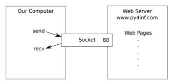
Once we send that blank line, we write a loop that receives data in 512-character chunks from the socket and prints the data out until there is no more data to read (i.e., the recv() returns an empty string).
