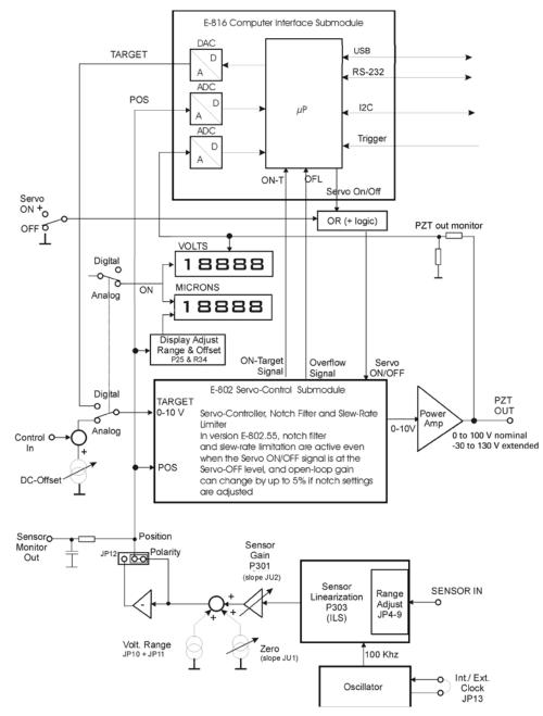
Fig. 5: E-665.CR block diagram
