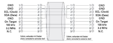
Abb. 15: E-625.CN network cable for networking of E-625.CR with E-665.CR
