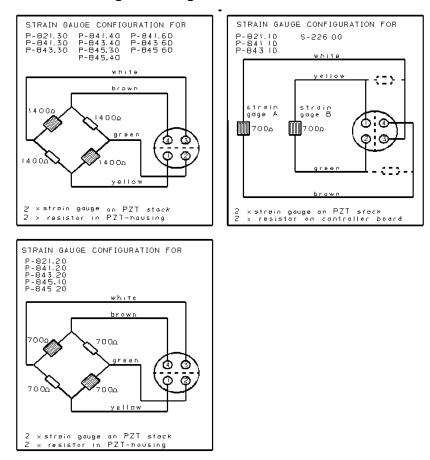
Fig. 12: SGS sensor wiring with various PI stages
