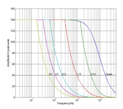
Fig. 11: E-665 open-loop frequency response with various PZT loads. Capacitance values are in  $\mu$ F.
