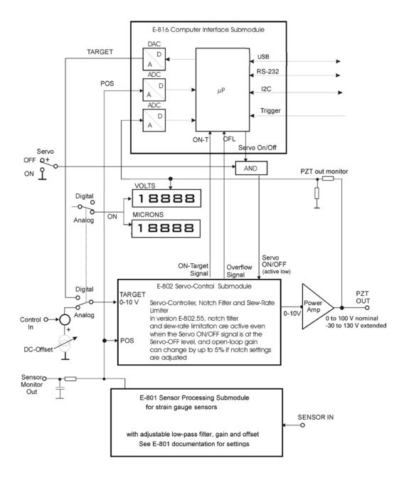
Fig. 6: E-665.SR block diagram
