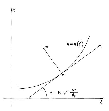
Figure 11 Propagation of Plate Error to the Trace
