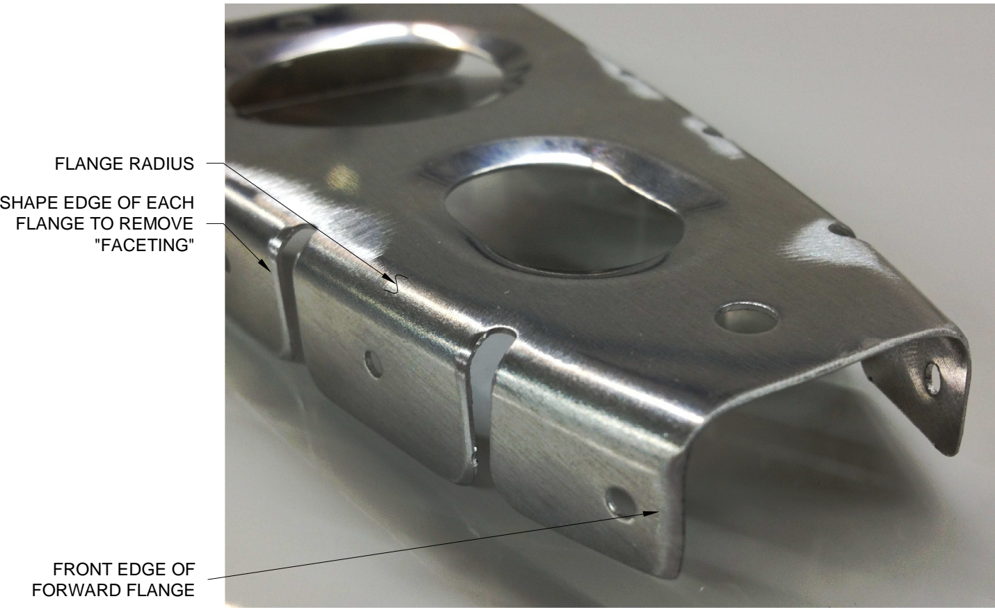
FIGURE 3: RIB FLANGE PREP
