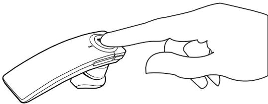
To switch the Q1 on or off, hold down
