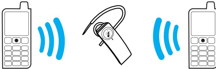
The Q1 supports **multipoint technology**. This means that you can use one Q1 headset with two different mobile phones or Bluetooth devices at the same time: if either phone rings, you can answer it with the Q1.
