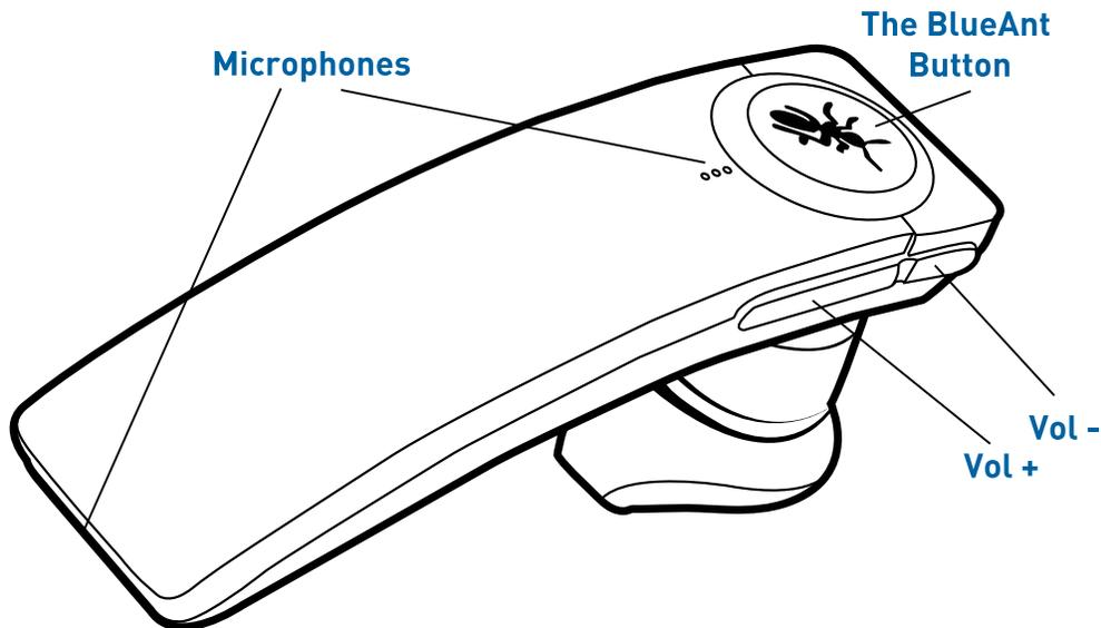
In addition to the volume up and down buttons, the Q1 has a multi-function button called the BlueAnt button. You use this to turn the Q1 on and off and to activate the voice recognition. You can also access some advanced functions by pressing different combinations of the three buttons. For a full description of all the button functions, see ["Button Functions" \(page 37\)](#).
