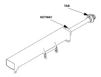
Q130 Water Distribution Tube Disassembly
