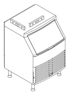
**Checking Ice Machine Level**
