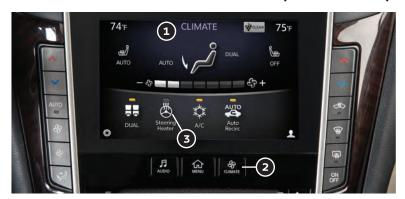
The climate controls can be adjusted using the buttons on either side of the lower display or through the "CLIMATE" screen (1) on the lower display.
