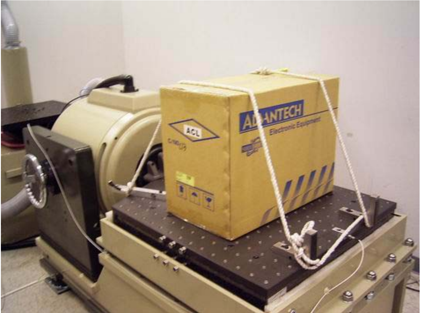
IPC-7220 package vibration test for X-axis
