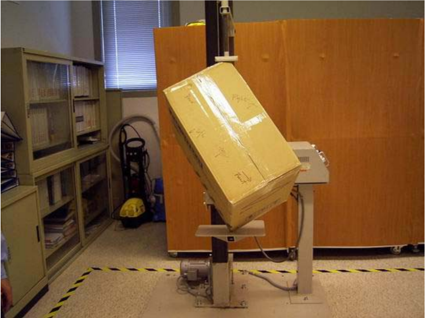
IPC-7220 drop test for one corner
