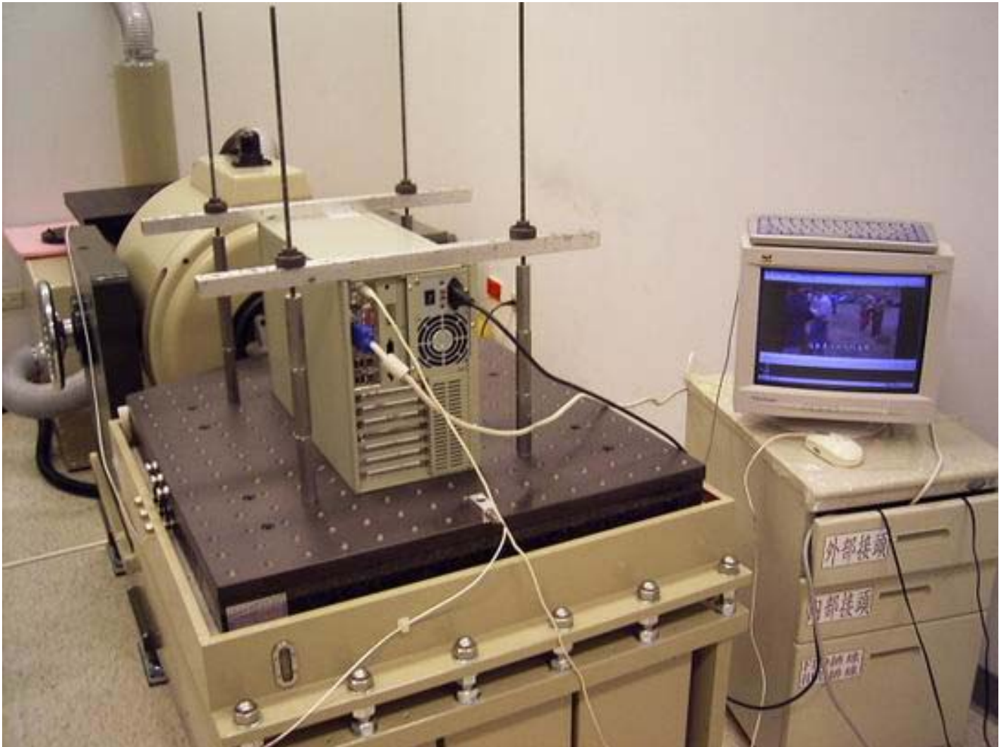
IPC-7220 random vibration test for Y-axis
