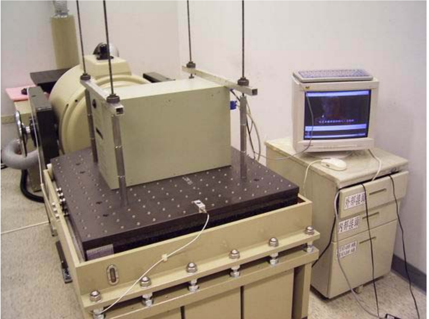
IPC-7220 random vibration test for X-axis
