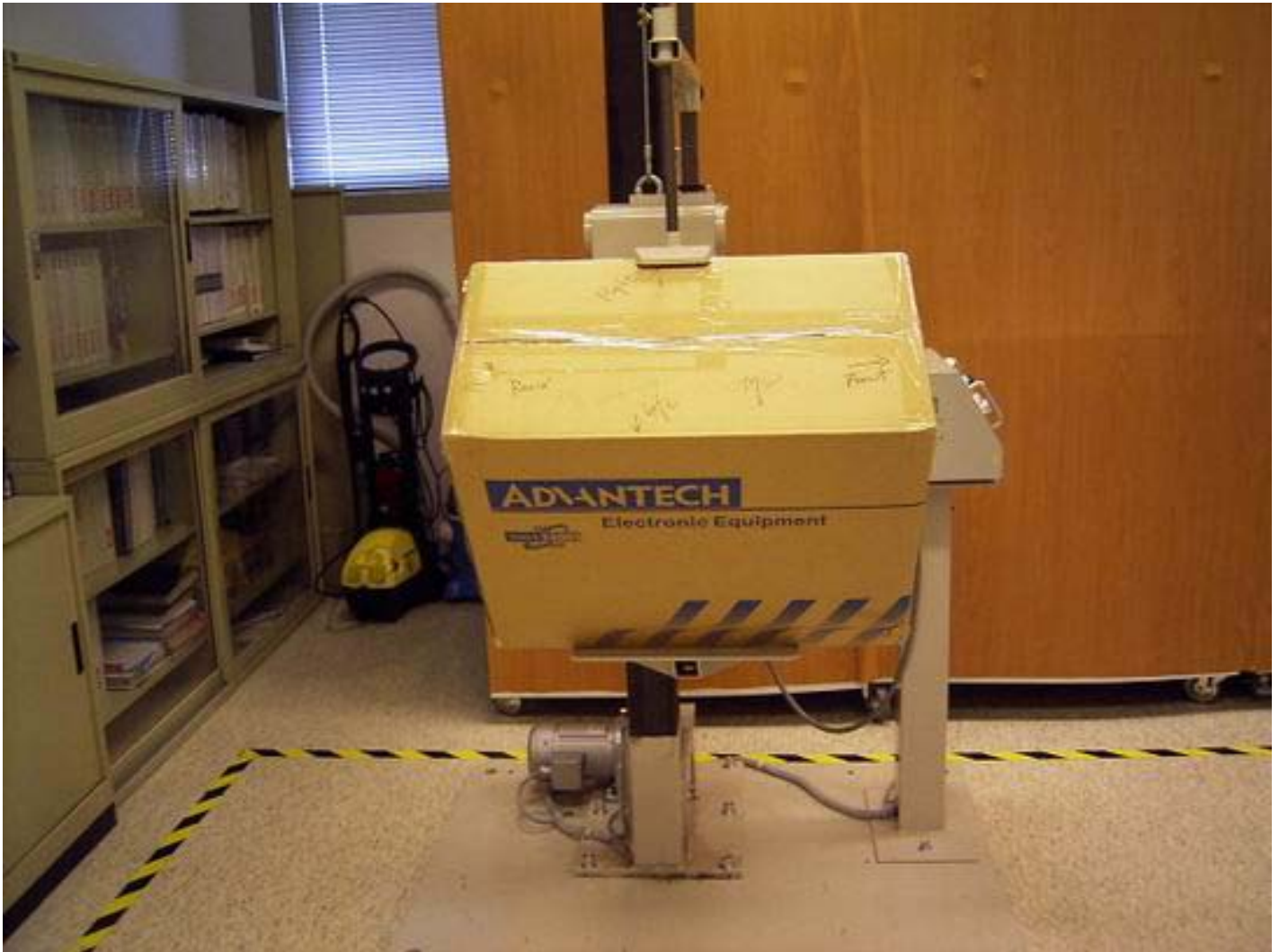
IPC-7220 drop test for three edges
