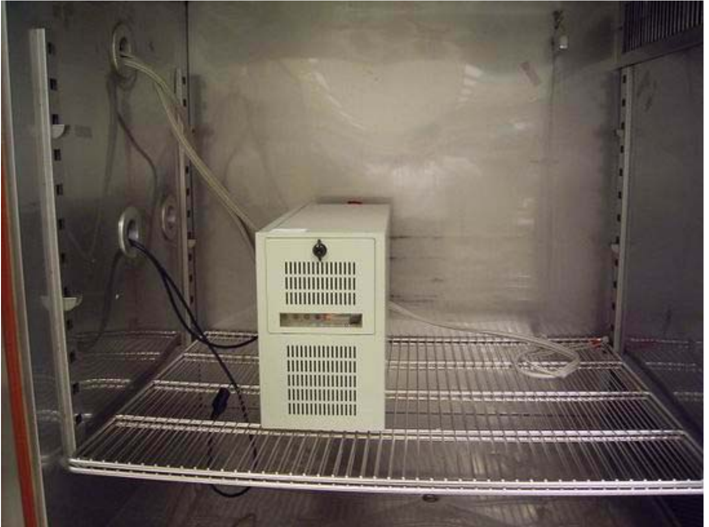
IPC-7220 high temperature operation test
