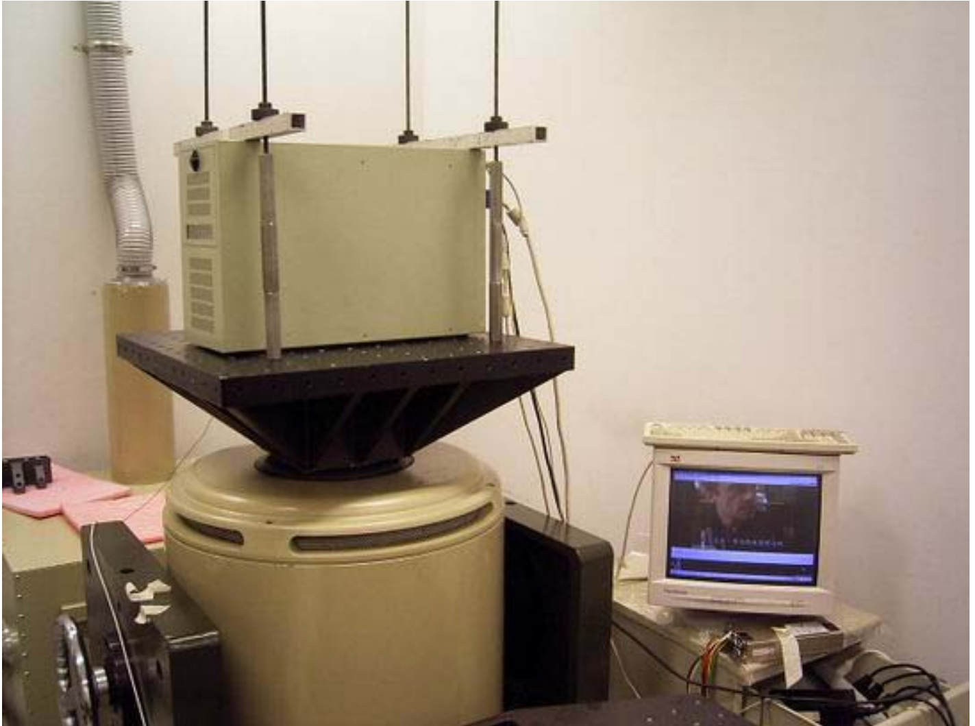
IPC-7220 random vibration test for Z-axis
