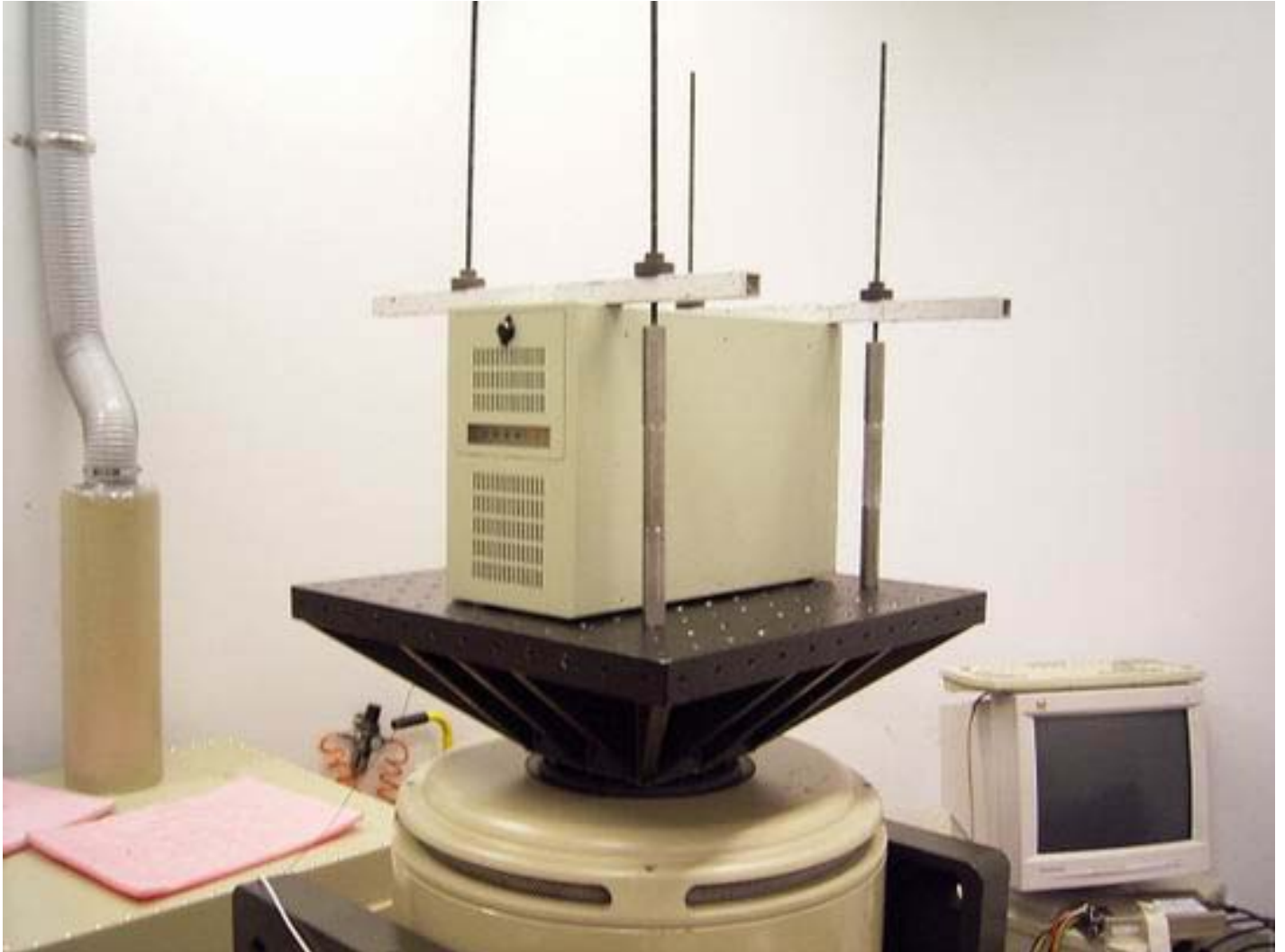
IPC-7220 sine vibration test for Z-axis
