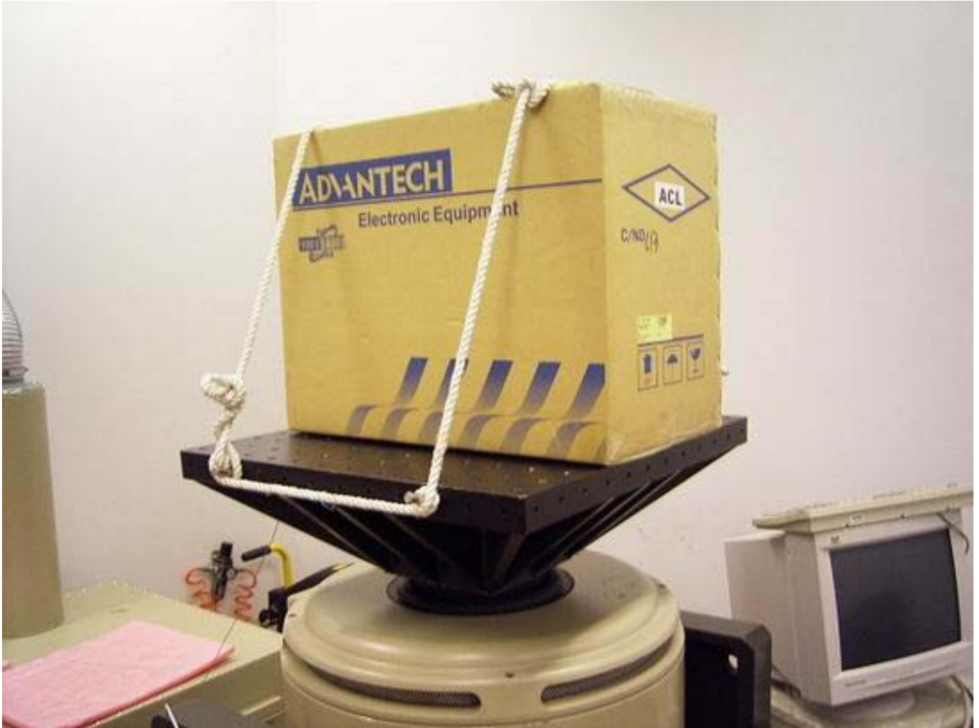
IPC-7220 package vibration test for Z-axis
