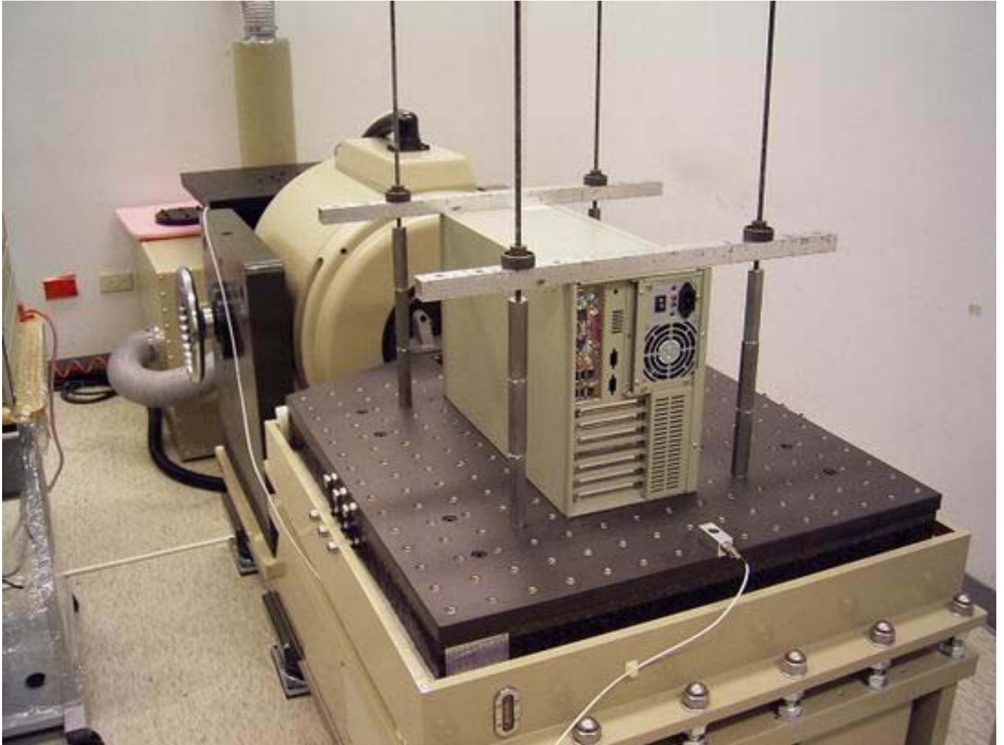
IPC-7220 sine vibration test for Y-axis
