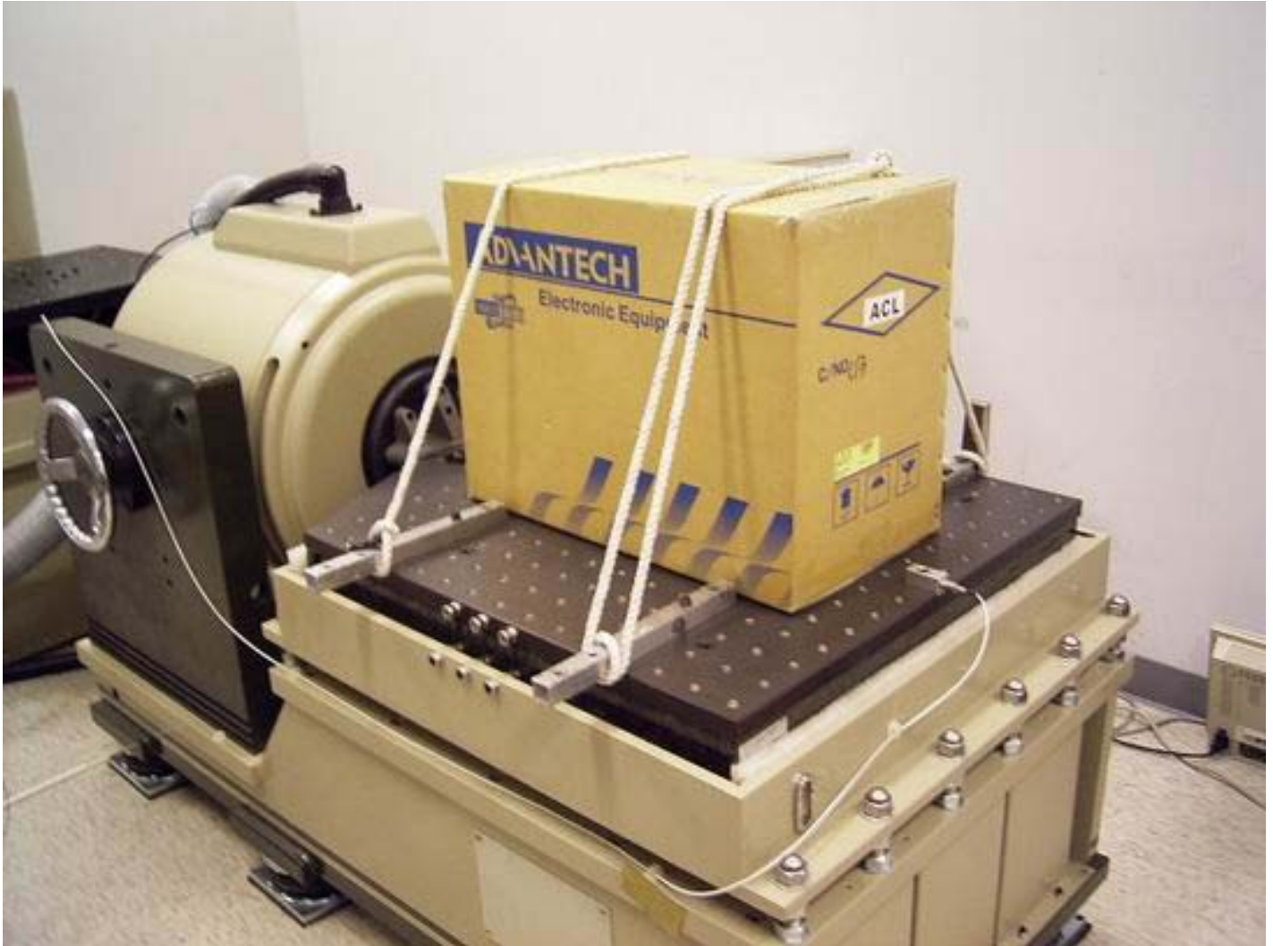
IPC-7220 package vibration test for Y-axis
