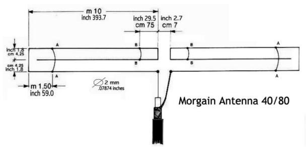
This antenna originally designed in the U.S. was born as an antenna for 40 and 80 meters and has been adapted for 20 and 10 mand can have excellent performances on the 15 meters, with a total length of 20 meters.
