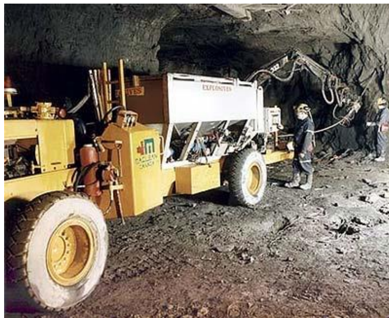
Figure 4: Underground emulsion vehicles with control operator and observer.
