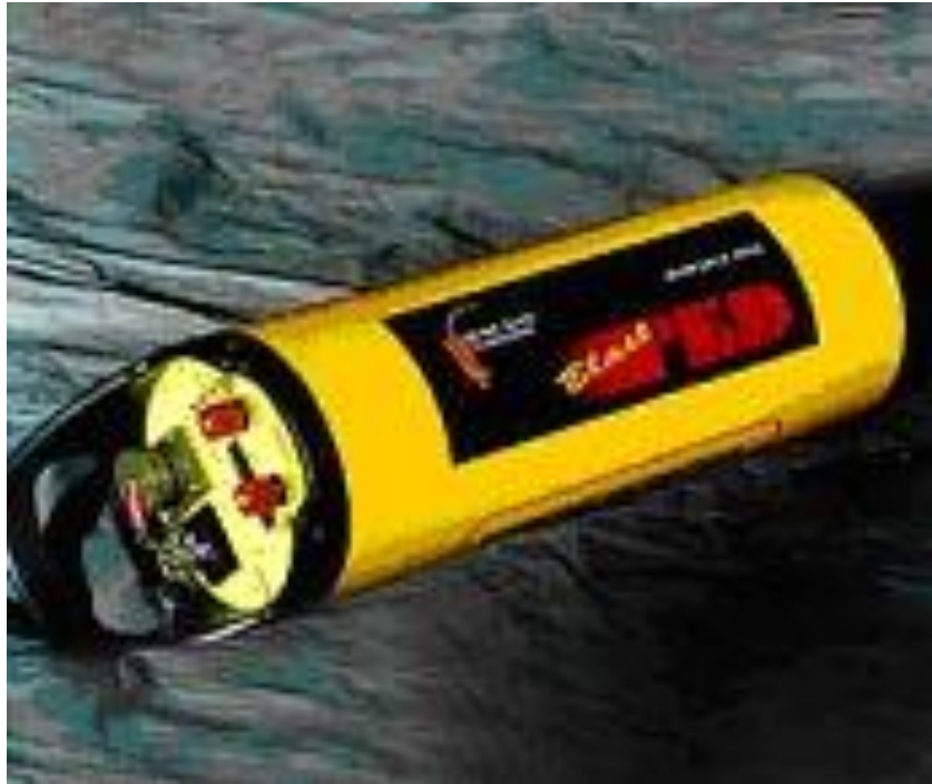
Figure 5: Underground remote blasting using BlastPED system.
