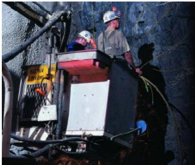
Figure 3: Charge car basket with receptacles for explosives
