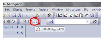
Zoom the filter image and define a polygon by using the HREM Polygon ROI tool. At first select the Polygon ROI, and click the first point, then move the mouse pointer to the next point and click to fix the second point. In this way, you can define the polygon of any number of vertices. Press double click when finished. The polygon will be drawn in green. If you make any error in the polygon definition, you can delete it (*Select* the ROI and press *Delete* key).
