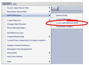
The second operation is the calculation of a new histogram of all maxima found in the Cross-Correlation map between the *Refined* motif and the original image. The HREM Histogram tool and a new histogram window will appear. Usually, the cross-correlation values are in the range 0.7-0.9. If you want, you can change the histogram range as well as the number of bins. When you change these values, push the "Apply" button.
