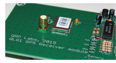
lower end of L3, to the SMA centre connector. This arrangement supplies power to the external antenna, from the RF Vcc supply output of the RF module. Note that it does not have short-circuit protection!
