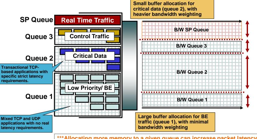
\*\*\*Allocating more memory to a given queue can increase packet latency, which could impact application performance.
