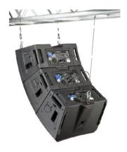
KLA offers solutions for both permanent and temporary suspension. For permanent installations each element has four M10-threaded points on the top of the cabinet, and one in the bottom center of the rear of the cabinet for aiming.
